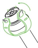
Pull one of the strap ends over a sensor mount wing, using the top hole in the strap. Pull each of remaining two strap ends on the respective sensor mount wing.
