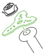
Place the end of your bat on a firm surface with the knob pointing upward. Stretch the round hole in the center of the sensor strap over the knob. Position the sensor mount on top of the bat knob. Hold the sensor mount in place with one hand.
