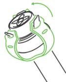
Pull one of the strap ends over a sensor mount wing, using the top hole in the strap. Pull each of remaining two strap ends on the respective sensor mount wing.
